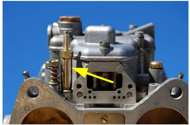
**Fig. 8** – Fitting installed – rear view
