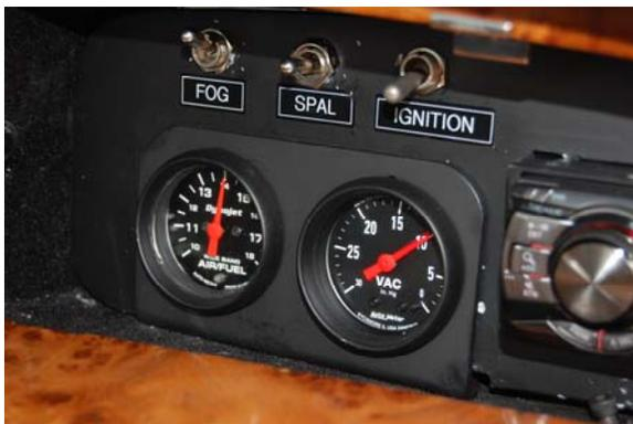
**Fig. 11** - AFR and manifold vac. gauges
