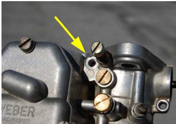
**Fig. 4** - Manifold vacuum access point
