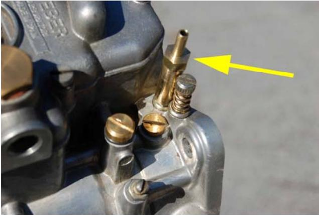
**Fig. 7** - Fitting installed – side view
