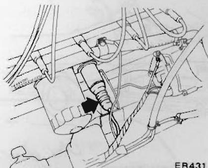
Fig. ER-11 Disconnecting wire for oil pressure sending unit
