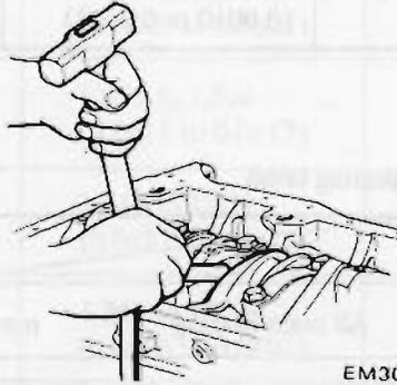
Fig. EM-65 Checking crankshaft end play
