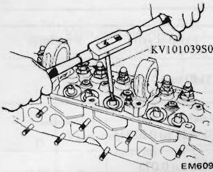
Fig. EM-44 Reaming valve guide
