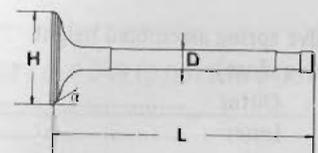
Fig. EM-36 Intake and exhaust valve dimensions
