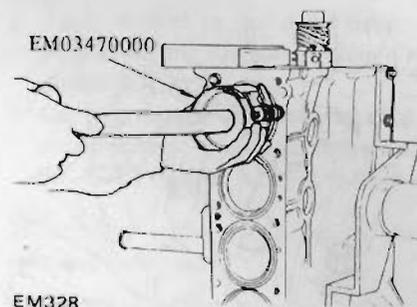
Fig. EM-96 Installing piston-rod assembly
