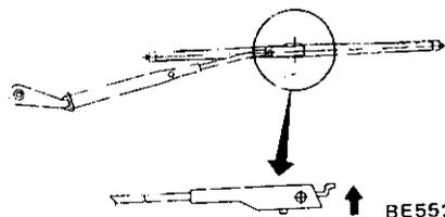
Fig. BE-110 Removing wiper blade
