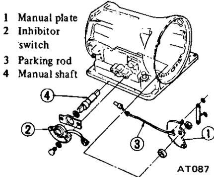
Fig. BE-43 Inhibitor switch
