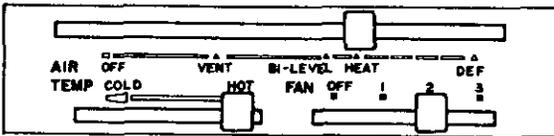
AIR lever is in HEAT position. TEMP lever controls temperature of discharged air. FAN lever controls amount of air discharged.
