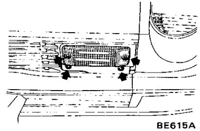
Fig. BE-27 Front combination lamp
