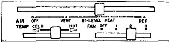
AIR lever is in BI-LEVEL position. TEMP lever controls the temperature of heat air discharged to floor or defroster nozzle. FAN lever controls amount of air discharged.
