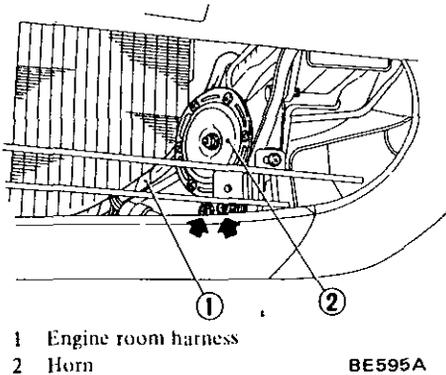
Fig. BE-104 Removing horn
