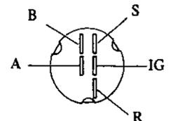
Fig. BE-45 Ignition and starting switch
