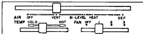
AIR lever is in VENT position. TEMP lever is in any position. Amount of discharged air is controlled by FAN lever. During high speed driving, FAN lever may be useless.
