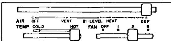
AIR lever is in DEF position. TEMP lever controls the temperature of discharged air. FAN lever controls amount of air discharged.
