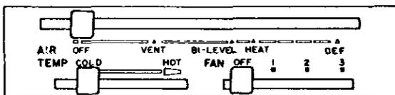
AIR lever is in OFF position. TEMP lever is in COLD position. FAN lever is in OFF position.
