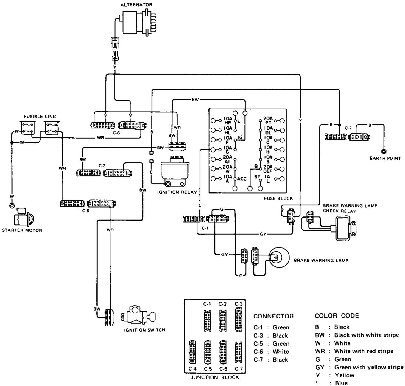
Fig. BE-54 Circuit diagram for brake warning lamp checking system
