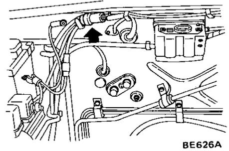
Fig. BE-111 Connector for wiper motor
