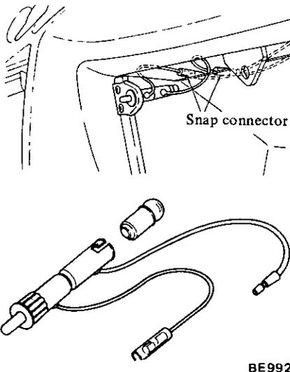
Fig. BE-35 Glove box lamp
