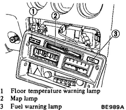
Fig. BE-33 Removing instrument finisher
