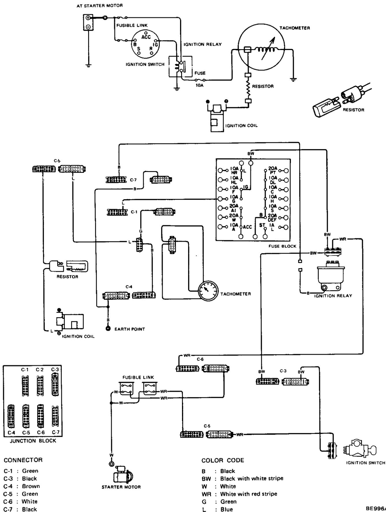
Fig. BE-50 Circuit diagram for tachometer
